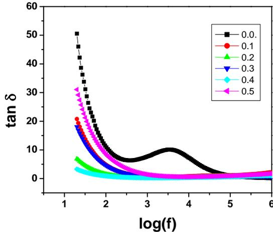
Fig. 3: Variation of loss tangent ( $\tan \delta$ ) of  $Mg_{1-x}Li_xFe_2O_4$  ( $0 \leq x \leq 0.5$ ) with  $\log(f)$ .
