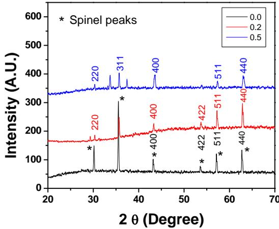
Fig. 1: X-ray diffraction pattern for the composition  $Mg_{1-x}Li_xFe_2O_4$  ( $0 \leq x \leq 0.5$ ).
