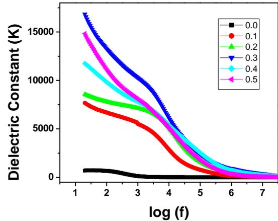
Fig. 4: Dielectric constant K of  $Mg_{1-x}Li_xFe_2O_4$  ( $0 \leq x \leq 0.5$ ) vs.  $\log(f)$  at room temperature.
